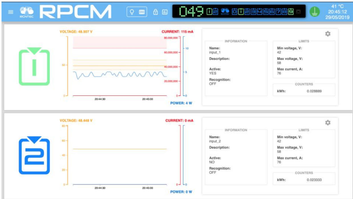
Figure 4.4.12. Showing Current Limits mode for the first input is on.
