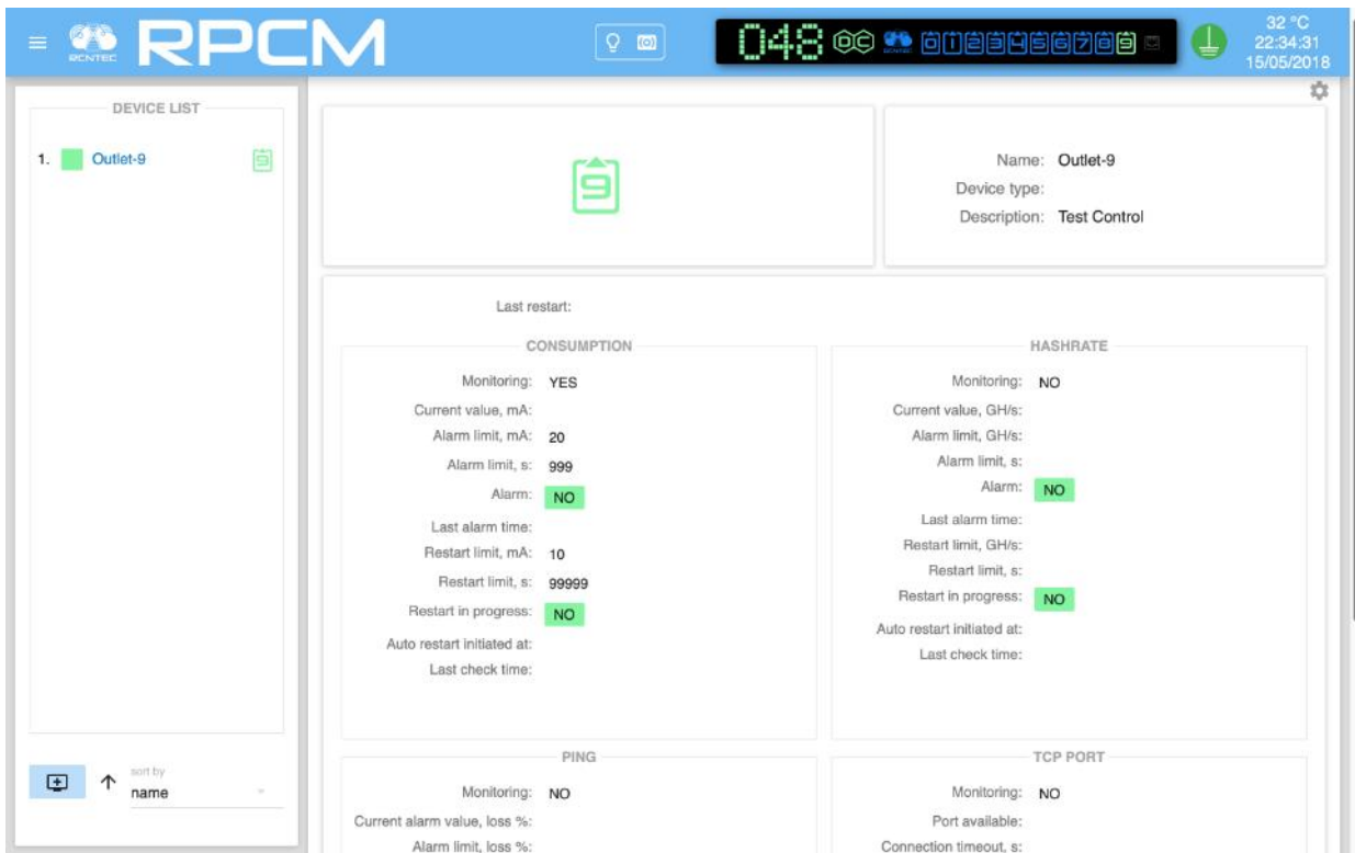
Figure 4.11.2. The Automation section window (PING, TCP PORT, and MINER STATUS subsections are not shown, scrolling is required).
