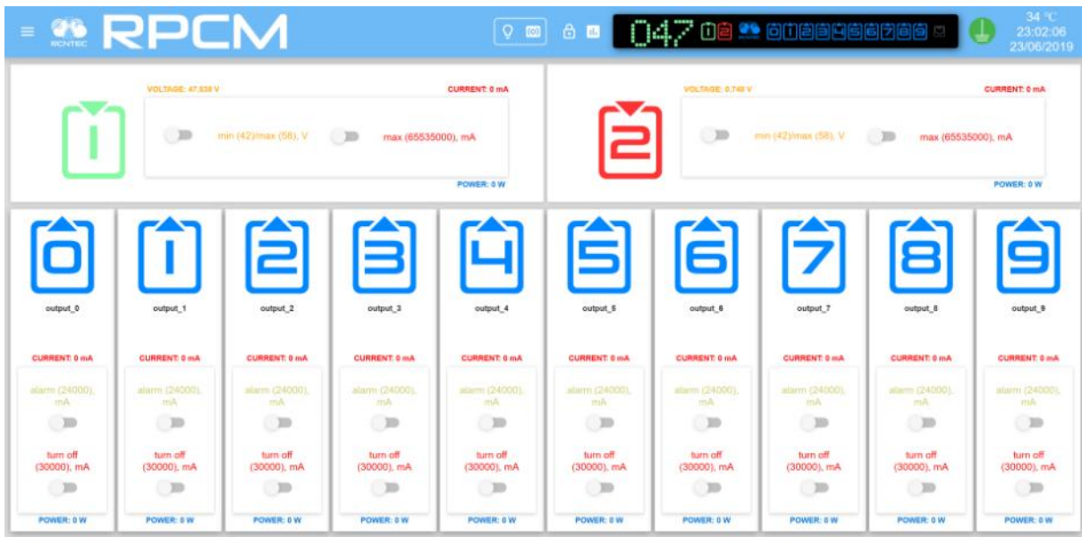
Figure 4.2.15. The Dashboard control panel in the Show Limits mode RPCM DC with ATS.
